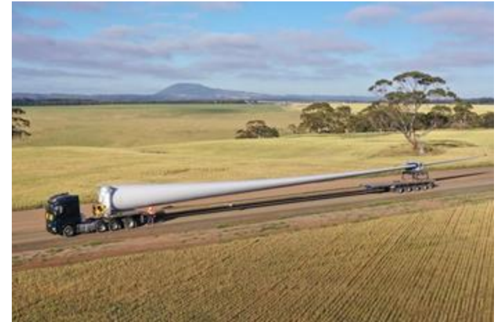
Transportation of 65m long turbine blade (2020)
