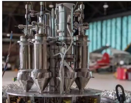
[ NASA and LANL's Kilopower ] <100 kWe
